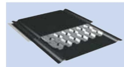
The turbulator, which controls the oil flow so that the maximum heat transfer is obtained, is designed for low oil pressure drop without the formation of a heat-insulating boundary layer in the oil tube.
