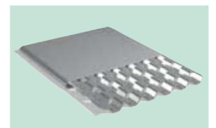
The turbulator, which controls the oil flow so that the maximum heat transfer is obtained, is designed for low oil pressure drop without the formation of a heat-insulating boundary layer in the oil tube.
