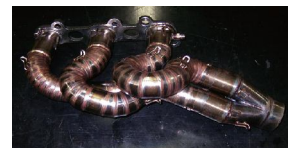
EQUAL LENGTH PROTOTYPE φ42.7 450mm
