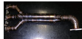
φ42.7mm BENCH DYNO TEST EXHAUST
