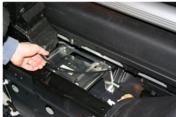
5.4) This shows the fish cable being routed from the location shown in picture 5.2
