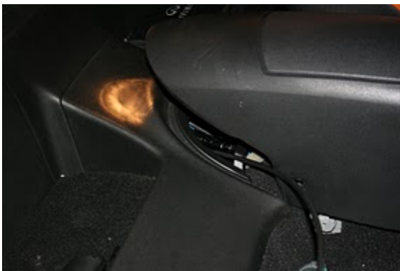
5.3) Once the center console/armrest is lifted up you can fish a cable to the trunk (shown in 5.4)
