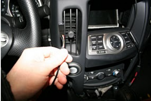
5.1) The connector above needs to be routed from behind the screen to the trunk
