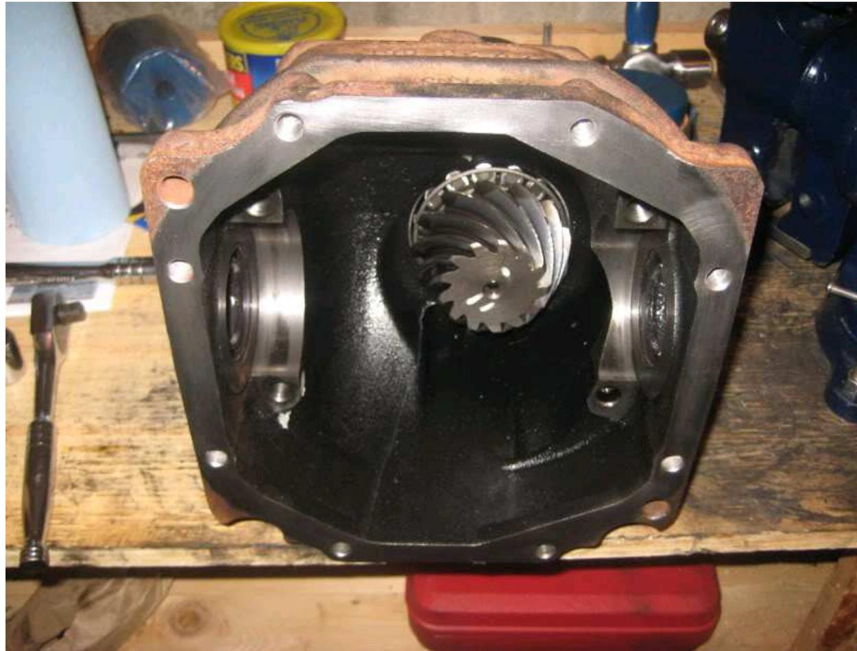
Place shims in appropriate locations with new bearing races.
