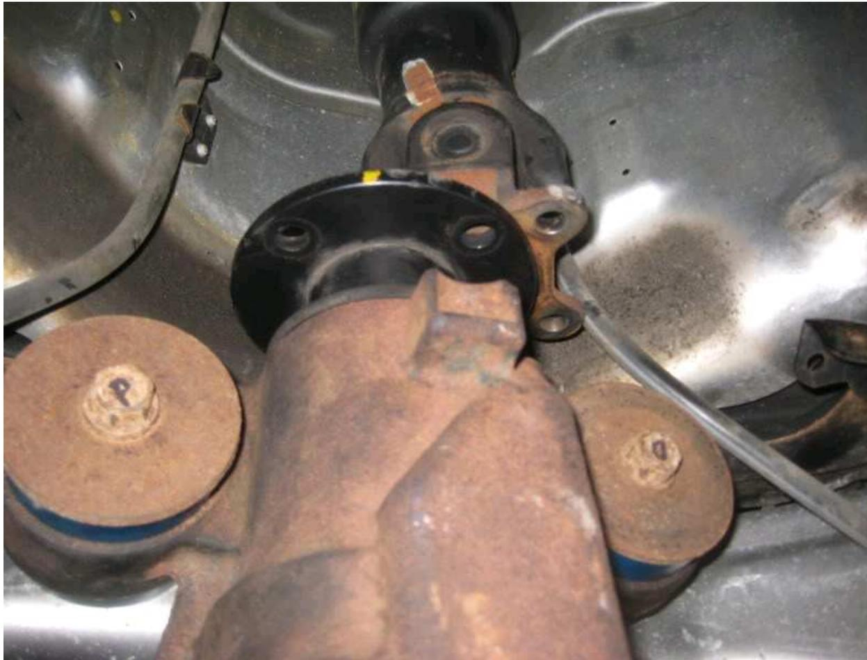
Torque the rear mount bolt to 74-88ft lbs and the 2 fronts to 67-81ft lbs, connect the wheel sensors.
