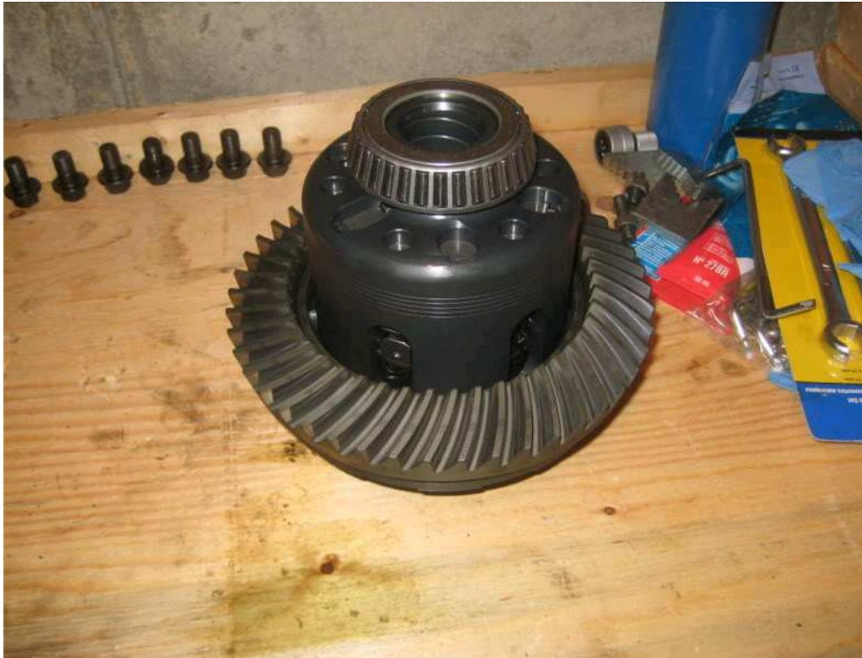
So at this point, Nissan recommends replacing all the ring bolt hardware and not re-using, I assume due to the stress on the bolts. I don't have them yet...so again it sits for now.
