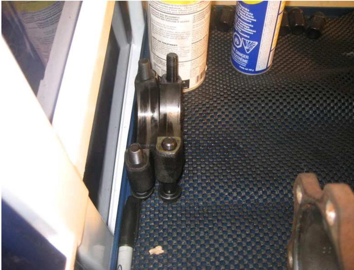
This was really tight (obviously) so I had to tap it out from the axle holes with a mallet and punch. Eventually I worked it out. If you care about your OEM VLSD then I would advise using brass drifts, or using a slide hammer to pull it out. I didn't care and you'll see later there is some damage on the inside from my use of cold steel punches.
