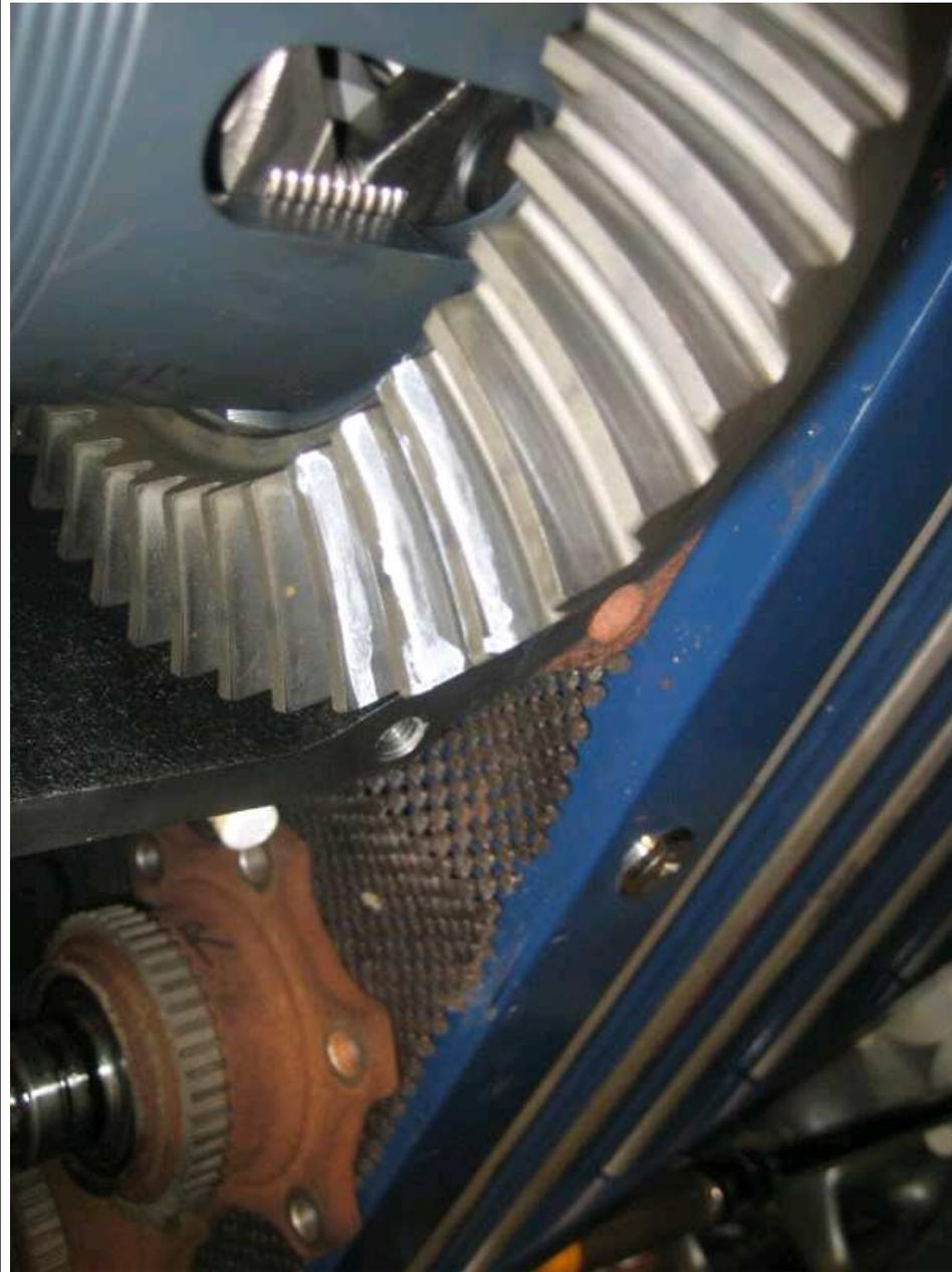
Each contacted correctly according to the manual...
