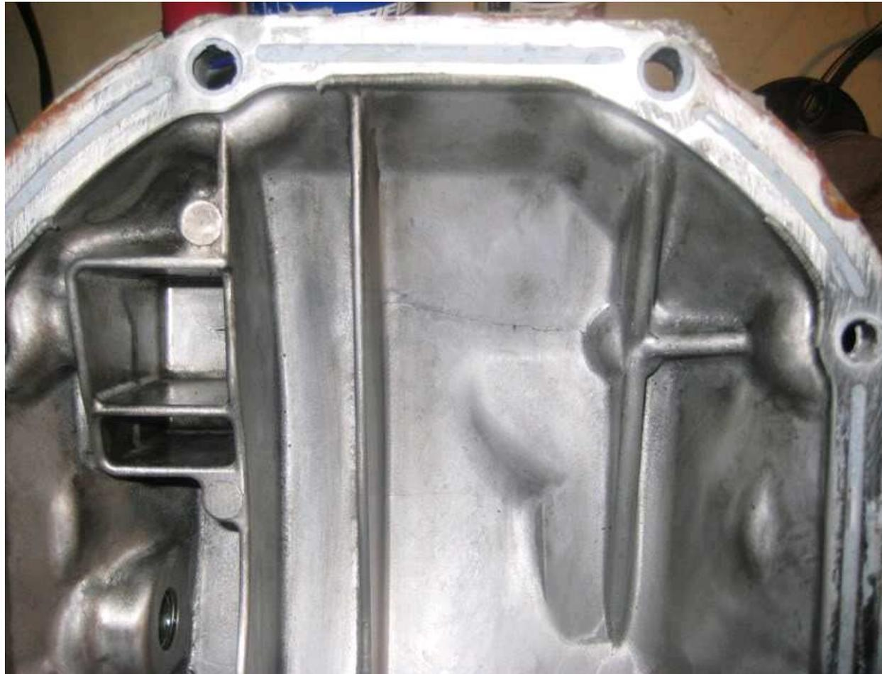
If I flip the cover around, that crack is stemming from where the rear sub frame mount is. But it's only on the inside...
