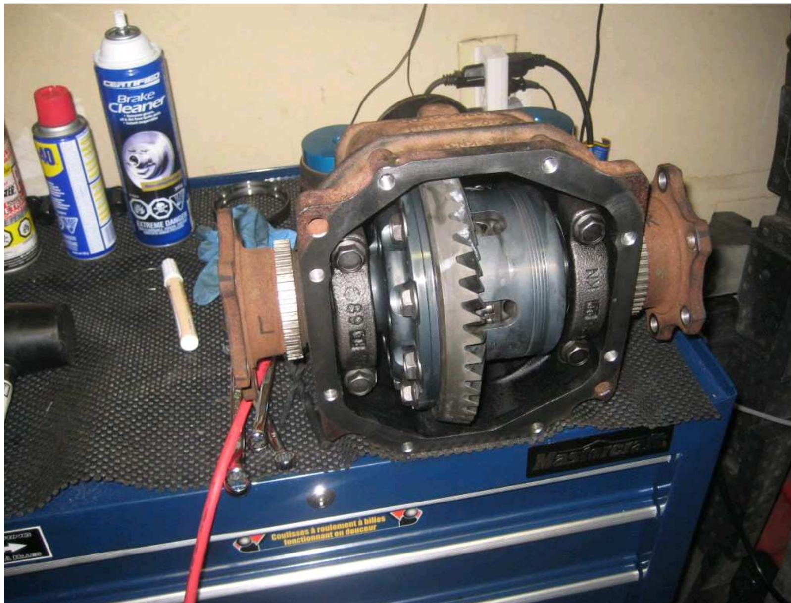
Using RTV high heat red, I made a gasket on the diff housing.
