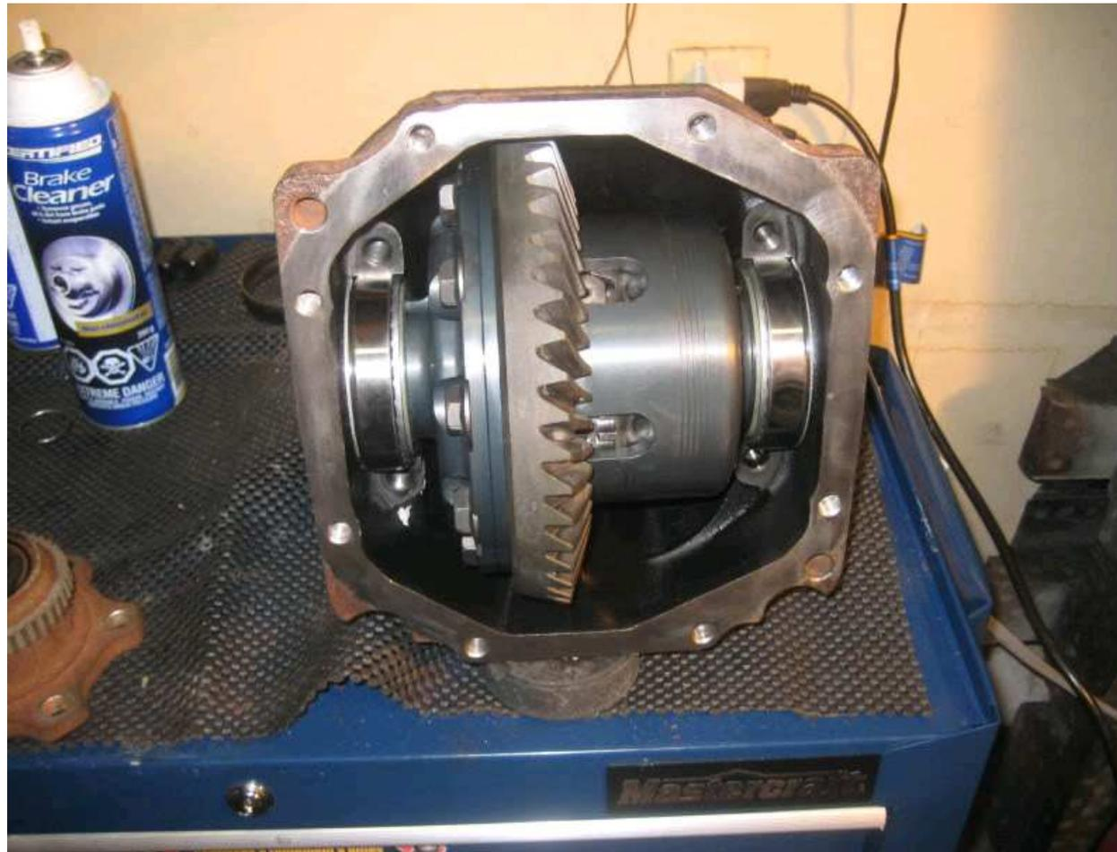
I placed the bearing caps on, and hand tightened the bolts. Then I torqued them in a criss cross pattern again to 65-72ft lbs.
