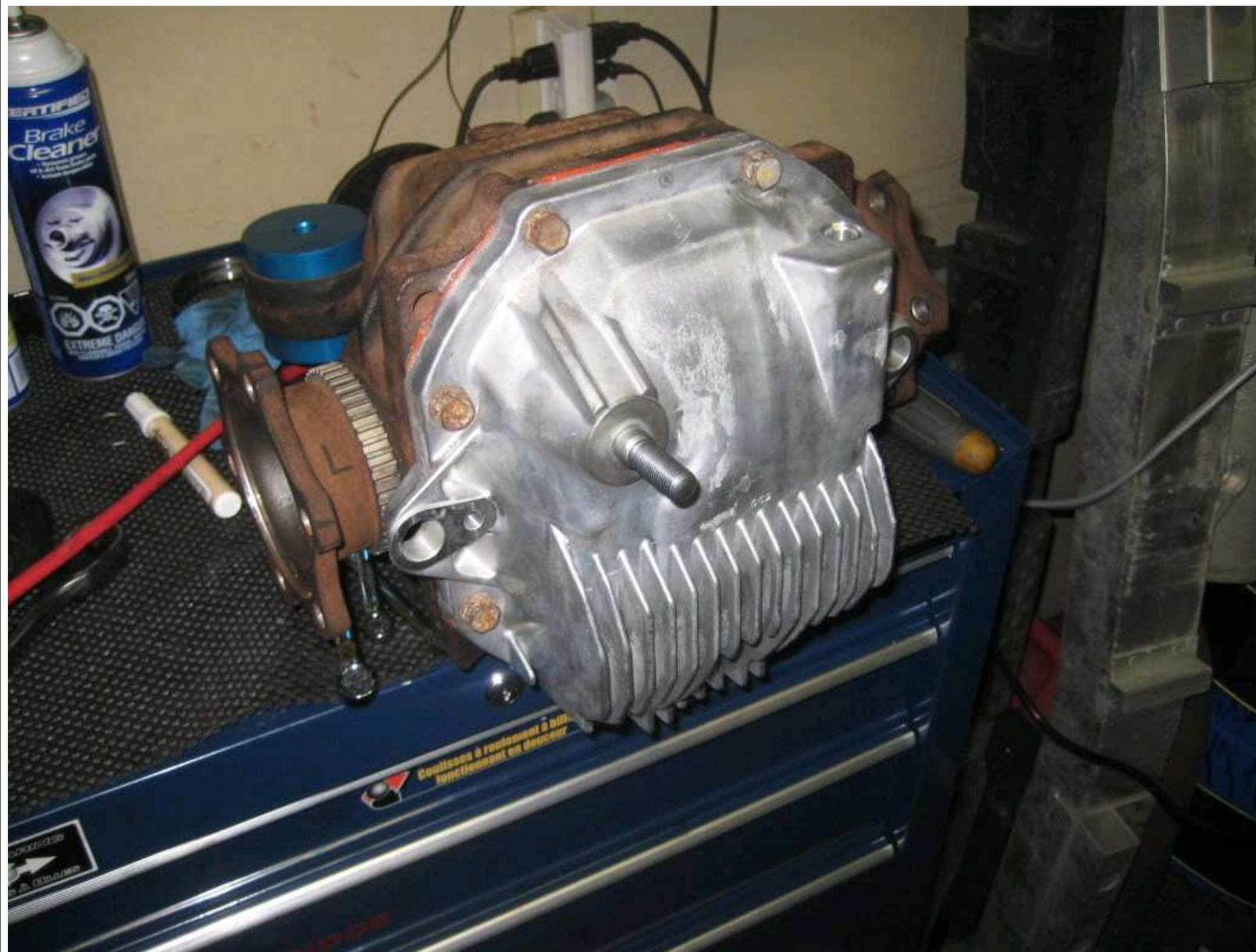
Installed Stud and wheels speed/ABS Sensor bolts and left it at that. I'll let the RTV cure, then dump some new fluid in it tomorrow...
