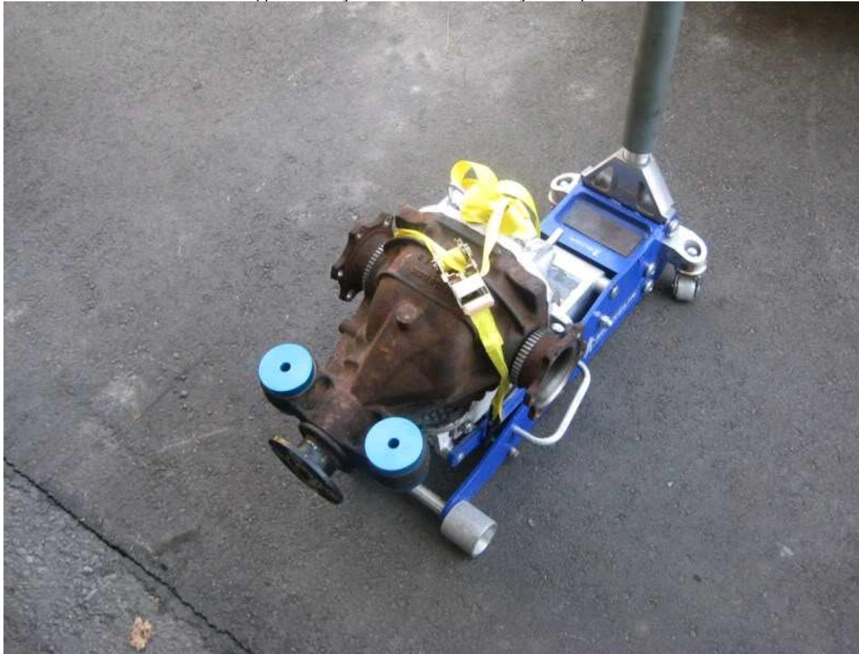
Oh to make my life a million times easier, something I should have taken the time to do in the beginning was remove the rear sway bar. This allows me to get directly under the car with the jack and lift it straight into place. With the sway in, I had to work it out over top...hindsight is 20/20, like a lot of things I learned during all of this.
