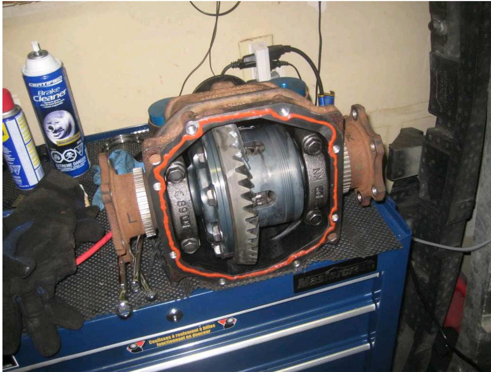
Torque the new cover on to 29ft-lbs using shitty old bolts, I should have bought new ones. Oh well.
