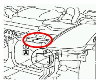
Remove a black plastic plate inside the marked area. This plate will block your air duct inlet. This is where the duct gets fresh air.
