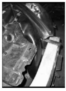
Slide the air duct tube from the top of the radiator support. This might be hard. You'll need to push in hard. Once it is placed. The top air duct inlet should be close to the air box (air duct inlet). Top of the EVO-R air duct tube has two screw holes. Line up with two screw hold marked below. Put the original screw back on and secure the air duct tube. The bottom part of the tube should be secure line up with the bumper support.
