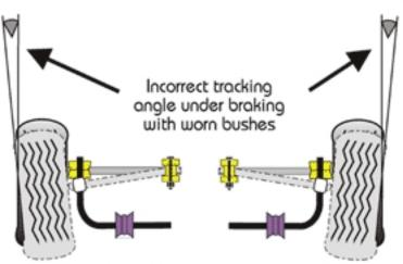
Old and soft rubber bushes cause incorrect geometry and excessive tyre wear as well as braking instability
